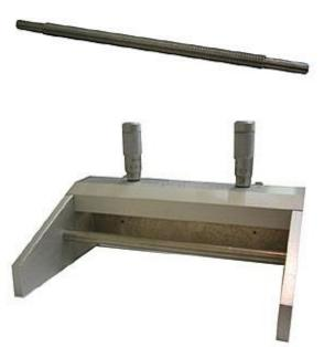
(Top) Wire Bar Coater : Stainless wire is wound onto 1/4 inch diameter stainless bar. Difference of wire diameter will produce different thickness of film.
