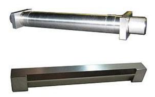
(Top) Baker type Applicator: Because the blade itself is eccentric, matching the right and left graduations with the guide line marked, the desired film thickness will be available. (0 - 10mil)
