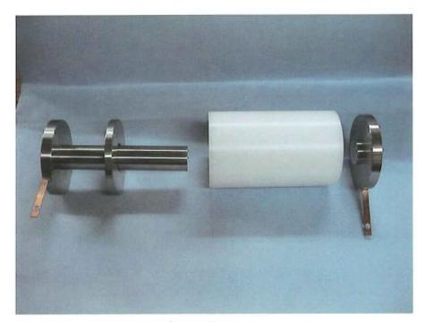
This cell is to analyze impedance of dry powder.
