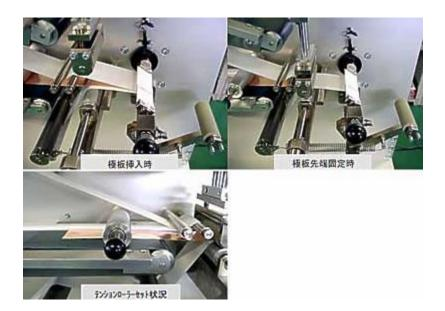
The electrodes are inserted and wound with tension from nip-rolls.
