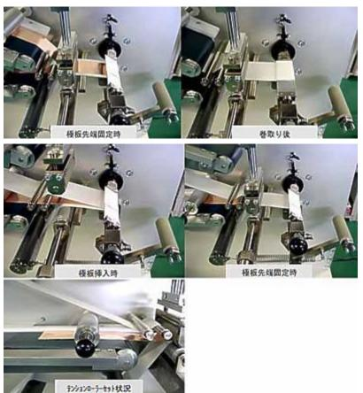
The separator is cut manually, and the mandrel is pulled forward and disassembled for the wound-electrode ejection.
