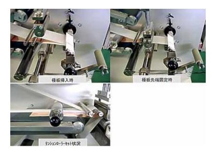
The electrodes are inserted and wound with tension from nip-rolls.
